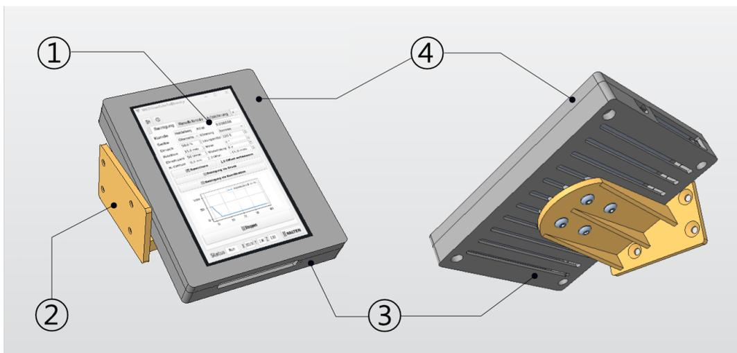
Figure 27: Operating and display unit of the robot
